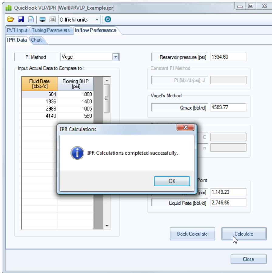
The routine will calculate the intersection point of the VLP and IPR relationships to give a resultant nodal analysis production rate and flowing bottom hole pressure.
